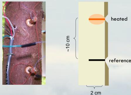
At night, sap flow is assumed to be zero. This yields our max  $\Delta T$ . During the day, as water travels up the stem, temperature ( $\Delta T$ ) varies with flow rate.
