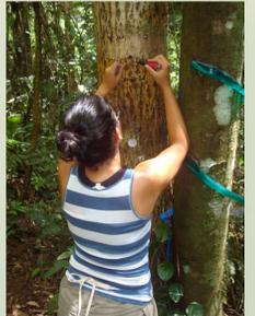
Figure 1. Granier heat dissipation sensors were installed into 15 trees. Sap flux velocities from the sensors were used to calculate transpiration rates.
