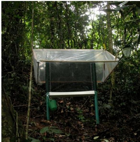
**Figure 3:** A Passive fog collector with rain awning.
