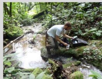
Figure 4: Testing for temperature and conductivity
