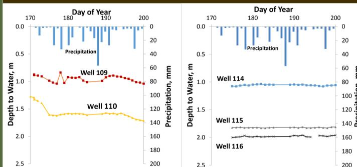
Figures 5 and 6: Depth to Groundwater for Upstream Series (left) and Trail Series (right)
