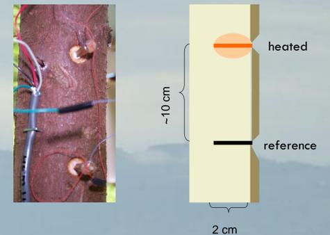
At night, sap flow is assumed to be zero. This yields our max  $\Delta T$ . During the day, as water travels up the stem, temperature ( $\Delta T$ ) varies with flow rate.
