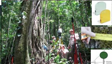
Terrestrial scanning laser (TSL) at 4-cm spacing, Stand Basal Area (Prism), DBH (tape), and tree height (laser hypsometer) data were acquired in a 30-m diameter stand plot on a 61 degree slope.
