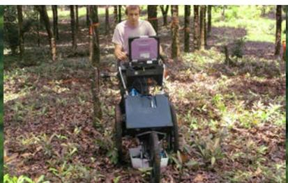
GPR data was collected in a 10-m X 10-m plot divided into 1-m X 1-m grids within the 30-m diameter stand plot. This data was collected at 400 MHz and 1.5 GHz.
